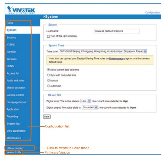
Each function on the configuration list will be explained in the following sections. Those functions that only show in Advanced mode are marked with Advanced mode. If you want to set up advanced functions, please click [Advanced mode] on the bottom of the configuration list to quickly switch to Advanced mode.
